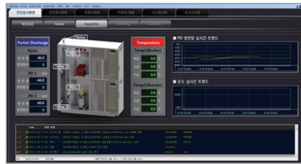
Switchgear Diagnosis (PD, Temp)
