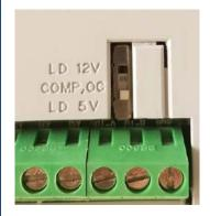
LD 12V = Line Driver 12VDC COMP, OC = Complementary/ Open collector LD 5V = Line Driver 5VDC
