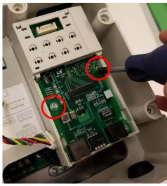
**Step 6:** Install the two screws to secure the Ethernet card to the standoffs. Snap the keypad adapter PCB into place on top of the Ethernet card.
