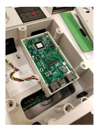
Step 5: Install the Ethernet card.
