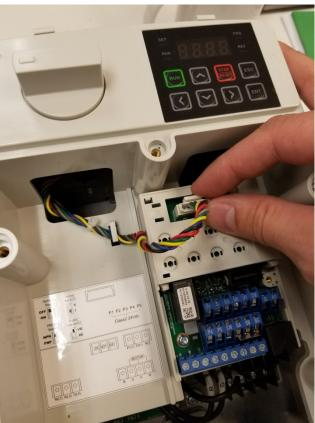
**Step 2:** Remove keypad connector.
