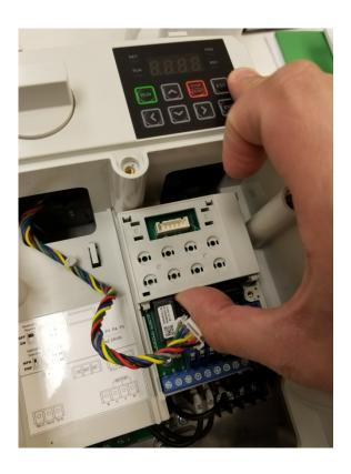
Step 3: Remove the keypad adapter PCB. It may be helpful to use a screwdriver to clear the plastic tabs.
