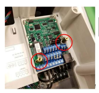
Step 4: Once the keypad PCB adapter is removed, install the two standoffs which are included in the Ethernet card kit.
