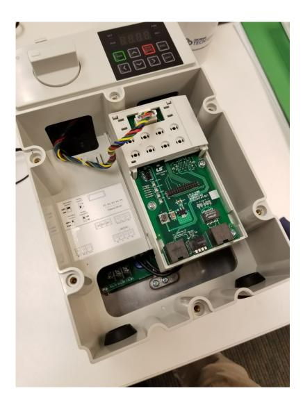
Step 7: Reconnect keypad connector cable. Connect network cable. Re-install front cover.
