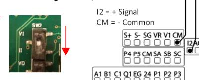
**Important:** Verify that SW2 dip switch on the terminal board to 'll' (down) for 4-20mA signal.
