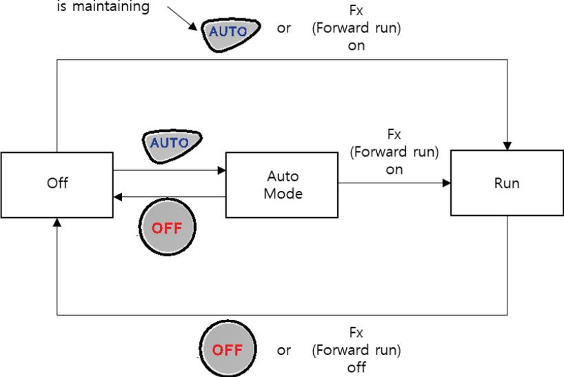
If [DRV-08 AUTO Mode Sel] is set to “1 (Disabled)”, the inverter automatically switches to AUTO mode and starts to operate when the operation command is input regardless of inverter’s state of being in AUTO or OFF mode.
