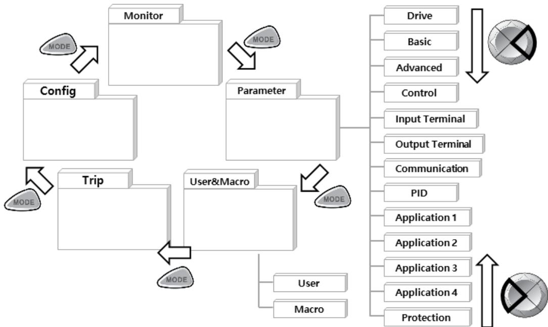
From the main screen, the [MODE] key will change the keypad to display the Parameter (PAR) mode. The PAR mode contains all parameters and monitors. These parameters and monitors are divided into intuitive groups. Pressing the LEFT or RIGHT arrows will move through the different parameter groups. While the UP and DOWN arrows will navigate through the different parameter code #'s in the selected group.
