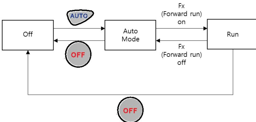
If [DRV-08 AUTO Mode Sel] is set to “0 (Enabled)”, the inverter starts to operate only when the operation command is input in AUTO mode.
