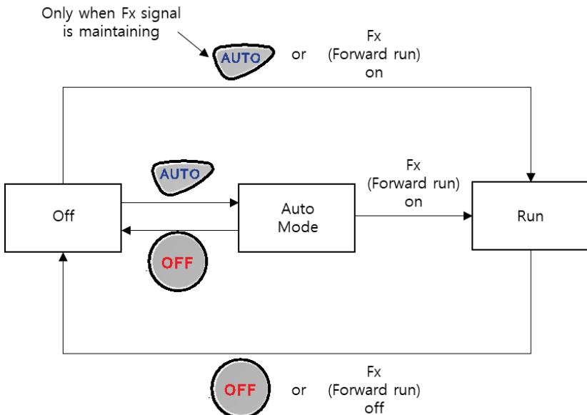
If [DRV-08 AUTO Mode Sel] is set to “1 (Disabled)”, the inverter automatically switches to AUTO mode and starts to operate when the operation command is input regardless of inverter’s state of being in AUTO or OFF mode.
