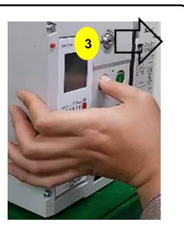
When the key is rotated to lock position, remove the key with pulling it
