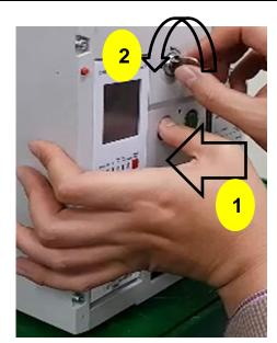
Turn the key CCW with keeping after pushing the off button
