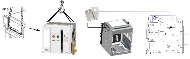
Fig. 2. Handling method of Fixed type
