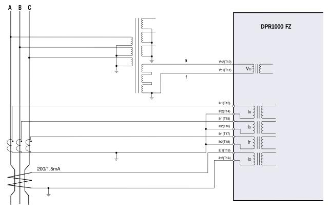
\*Take caution that in order to properly measure the phase, the polarity of zero phase voltage (Vo2, Vo1) and zero phase current must be set in the opposite direction
