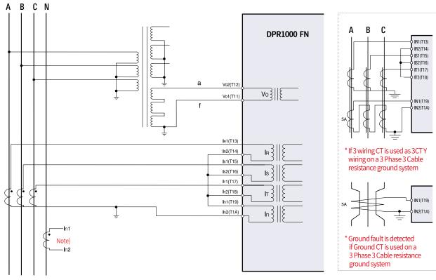
Note) When detecting ground fault using CT on the transformer neutral point ground wire, wire it with the ground wire
