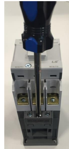
5. Replace 2 screws (be sure not to over tighten).
