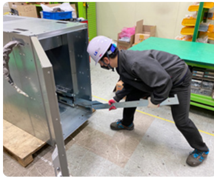
< Fig.8.2.3 Inserting extension rail >
